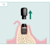
Cut healing plug. Ensure that no sharp edges remain that could irritate soft tissue.
