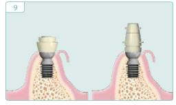
Place an emergence cuff or temporization sleeve onto abutment and modify, if necessary.
