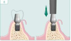
Use a template to confirm appropriateness of abutment prior to engagement of locking taper connection, then tap on abutment in long axis of abutment post to engage locking taper.
