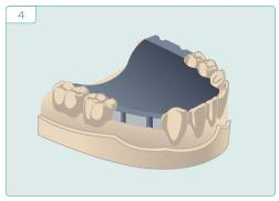
Cut a 2.5mm wide groove in the acrylic corresponding to the middle of each intended tooth to be replaced.
